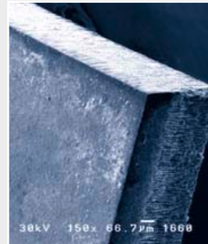
Precise cuts in sensitive materials (aluminum nitride).
