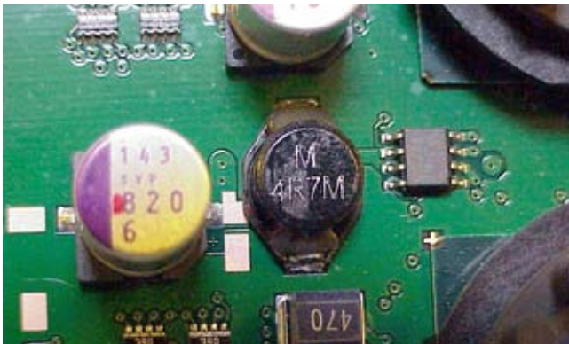
Removal of solder-resist on an assembled PCB
