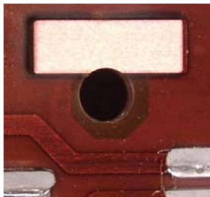
Polyimide cover foil opened on an assembled rigid-flex PCB
